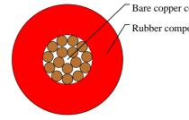
Bare copper conductor Rubber compound insulation
